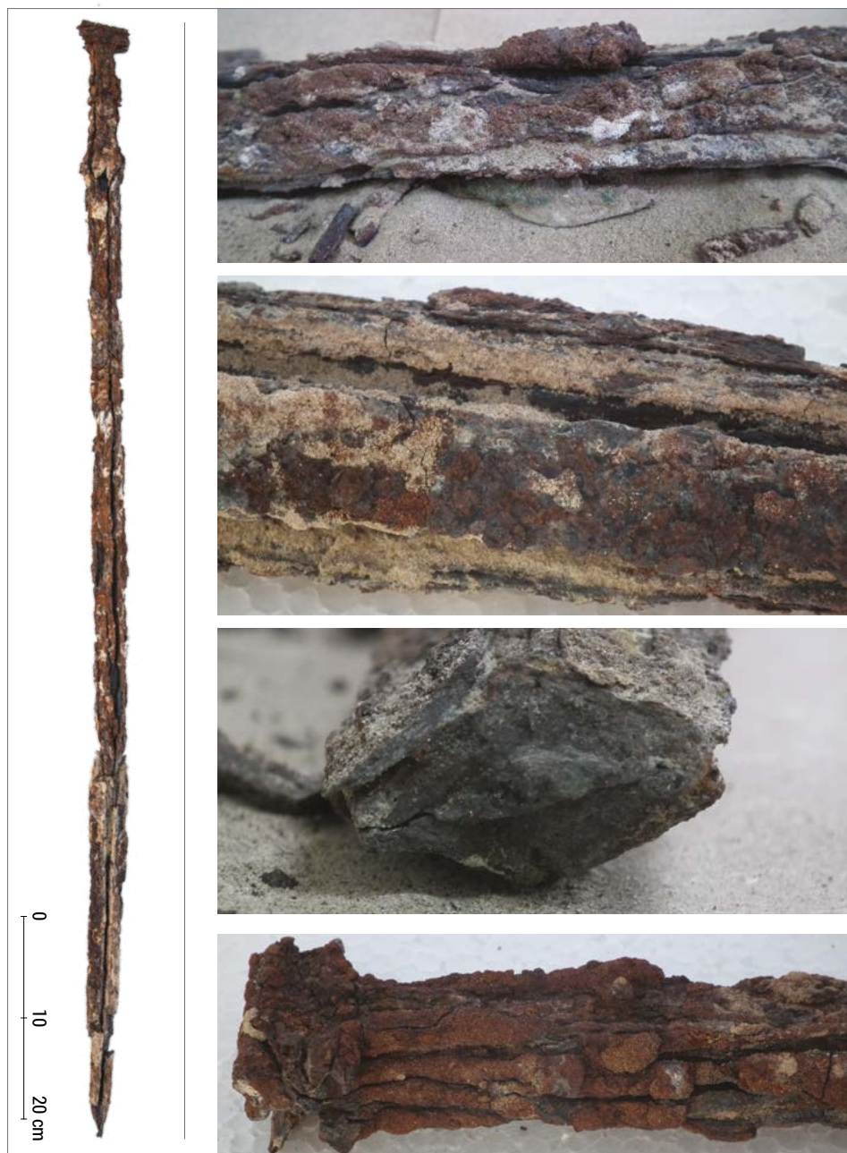
Fig. 11. Iron sword SAH17-V8/6515/001: left, state after conservation; right from top, a – condition of the blade after discovery; b – another fragment of the same blade before treatment; c – section through the blade, after stabilization in alkaline sulphite solution; note complete absence of iron core; d – handle after stabilization, cleaning and consolidation. The degree of damage (deformation, numerous cracks) prevented a reconstruction of the original surface (PCMA UW PMSaruq Project, Dubai Municipality/photos W. Weker and J. Kurzawa)
