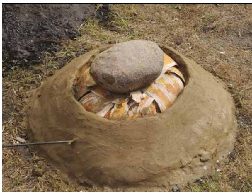
Fig. 2. Wood tar earthen pit during the filling and building of the dome (photo by K. Wasilczyk).
