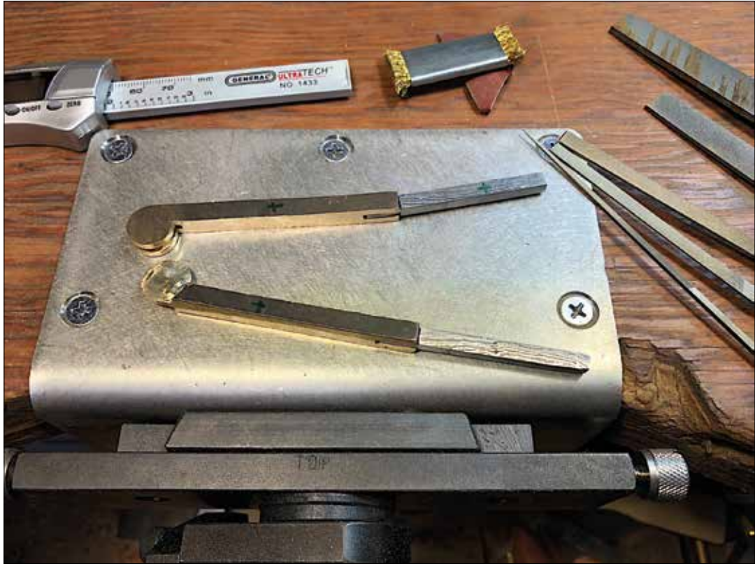
Fig. 6. Pair of brass and Damascus steel dividers in progress, during whitesmithing stage. (photo by Kent Heimer).
