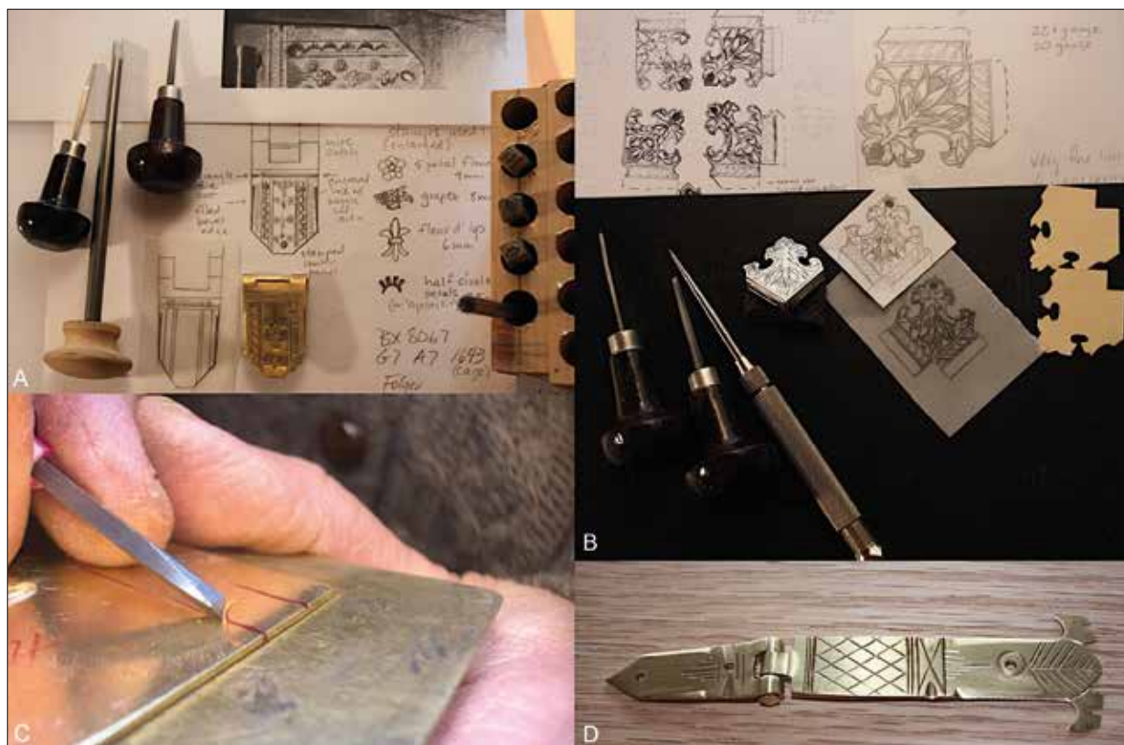
Fig. 4. A, B – patterns and tools used to scribe and engrave book furniture, with examples of formed and engraved work; C – close-up of engraving a line; D – common design of traditional book furniture forged at widest part, filed and engraved, hinge section formed and bent, stem riveted at both ends to prevent dislodgement in use (photo by Kent Heimer/Dawn Hoffmann).
