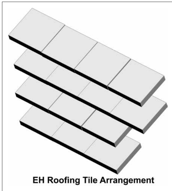
Fig. 3. A schematic representation of typical EH II ceramic roofing and the arrangement of these tiles on the roof (drawing by K. Jazwa).
