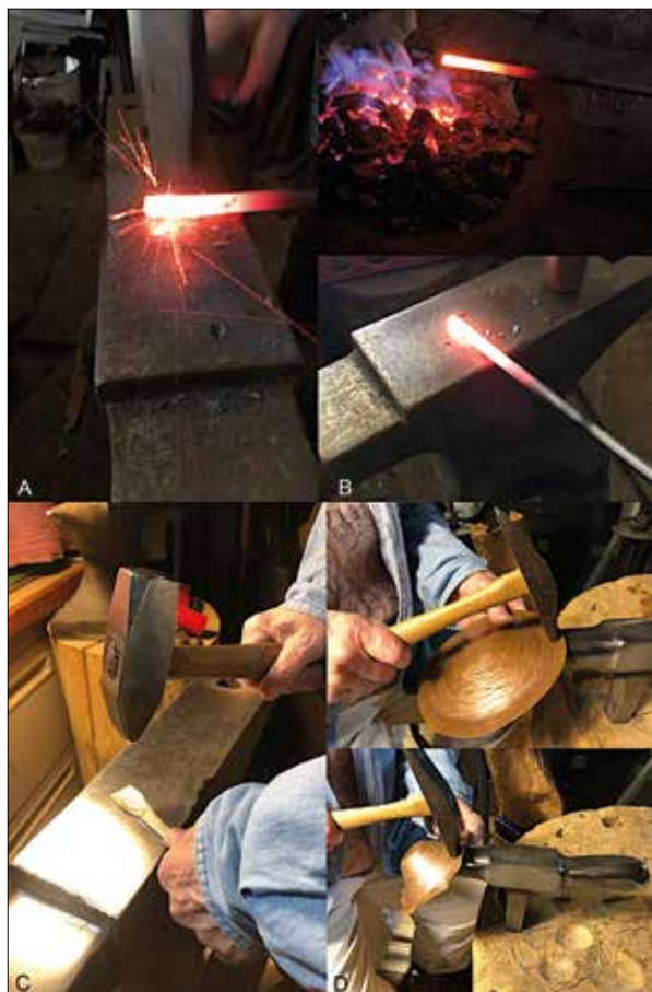
Fig. 3. A – hot forging iron at yellow-orange heat; B – iron in the coal fire and on the anvil before forging; C – cold forging silver using the cross peen face of the same type and weight of forging hammer to spread the metal (note the shinier anvil); D – two stages of raising a copper sheet over a T-stake using a cross peen raising hammer (photo by Kent Heimer/Dawn Hoffmann).
