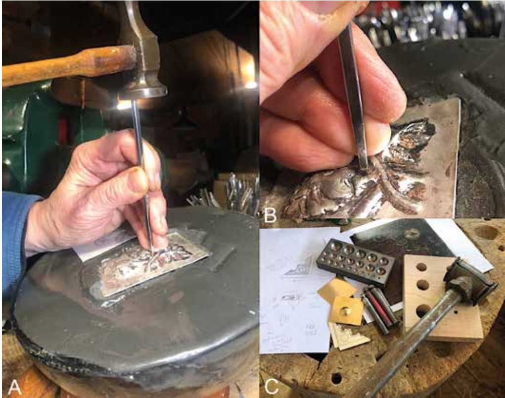
Fig. 1. A, B – adding chasing to a repoussé design, with pitch bowl supporting the work, using a hardened steel tool and metal surface; C – wooden and steel dapping blocks with punches, the resulting pieces are shown on the left-hand-side of the photo (photo by Kent Heimer/Dawn Hoffmann).
