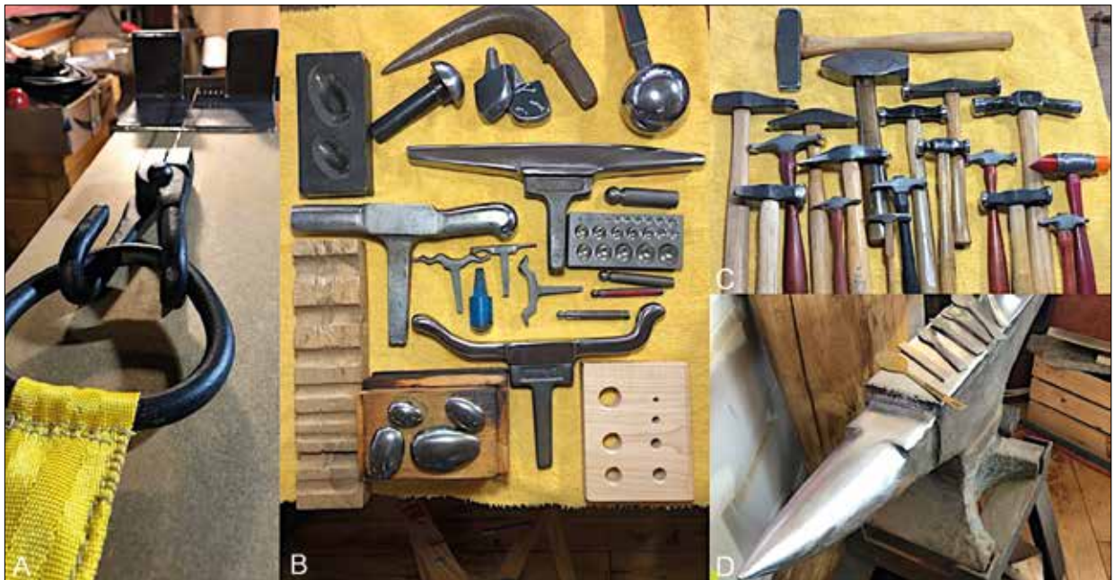
Fig. 2. A – drawing wire through a drawplate; B – various sizes of supporting T-stakes, mushroom stakes, wooden, steel and urethane forming blocks; C – a selection of various sizes and weights of hammers (all based on the traditional forging hammer with a cross peen and a round-faced hammer face); D – anvil for cold forging non-ferrous metals, samples show pattern and stages of making a spoon (photo by Kent Heimer/Dawn Hoffmann).
