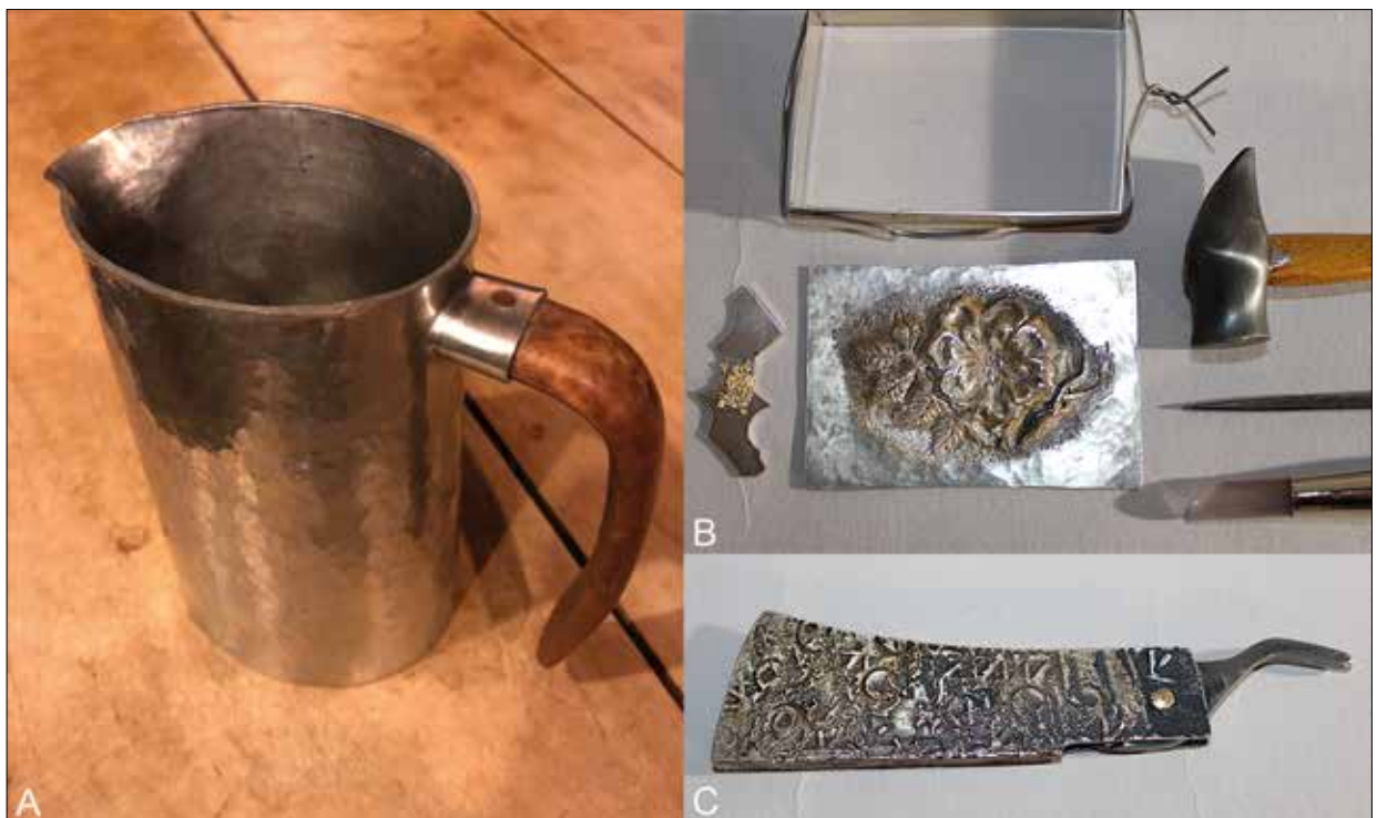
Fig. 7. A – pewter pitcher with riveted walnut handle; B – in-progress embossed silver box inlaid with gold, with wired lid awaiting brazing, embossed decorative top, required tools (hammer, chisel, agate burnisher) on right, and sample of gold onlay on left; C – folding knife with blade of Damascus steel and decorated sheath of iron and bronze (photo by Kent Heimer).
